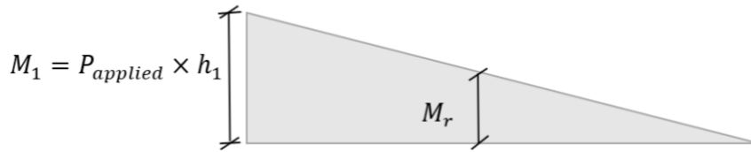
Figure 4. Required flexural strength M_r representation for calculation from moment diagram
