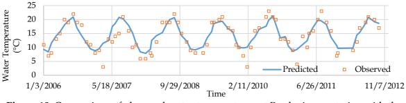
**Figure 10.** Comparison of observed water temperatures at Besdegirmen station with the simulated values predicted.
