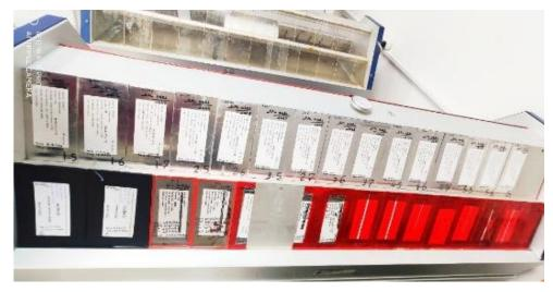
Figure 8. QCT test cabinet and the placed panels
