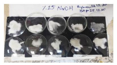
Figure 10. NaOH (25%) resistance test with the wetting method
