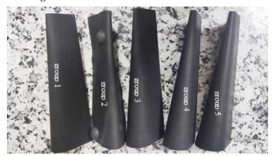
Figure 13. Results of the conical bent flexion test for the different groups of the study
